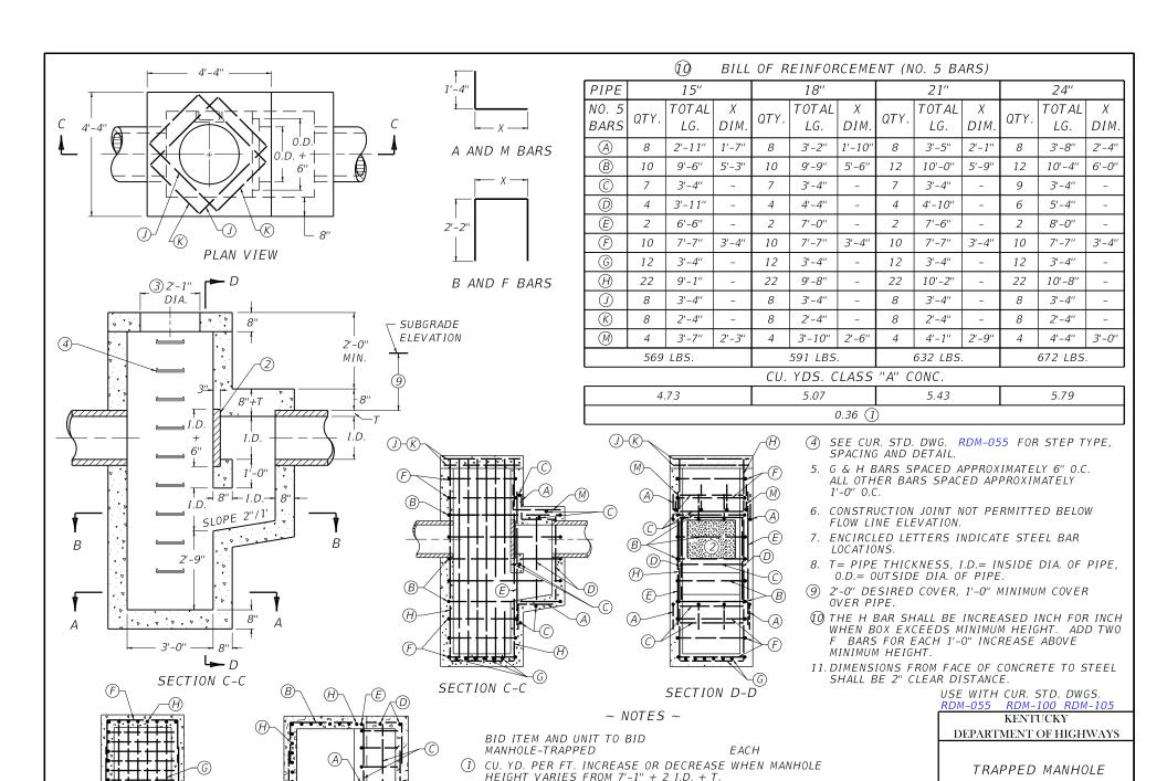
REMOVABLE STOPPER-MASONRY, CAST IRON OR OTHER TYPES OF STOPPERS WILL BE PERMITTED IF APPROVED BY THE ENGINEER.
